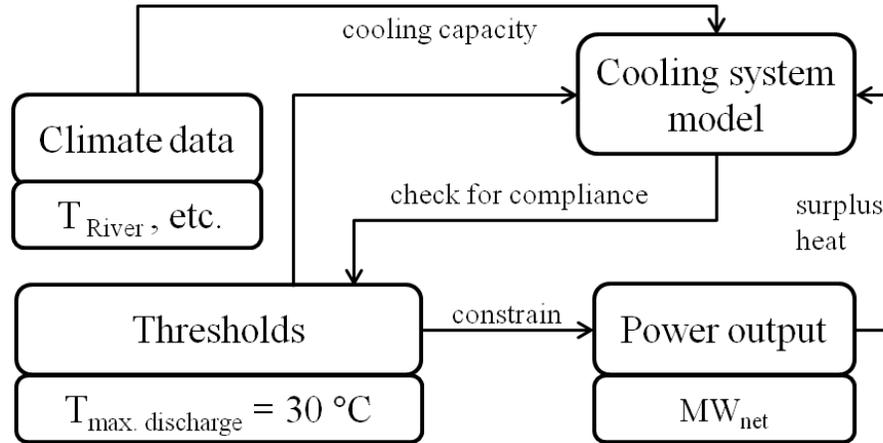
**Figure 1:** Schematic structure of a cooling system model with the most relevant components (Hoffmann et al. 2010)
